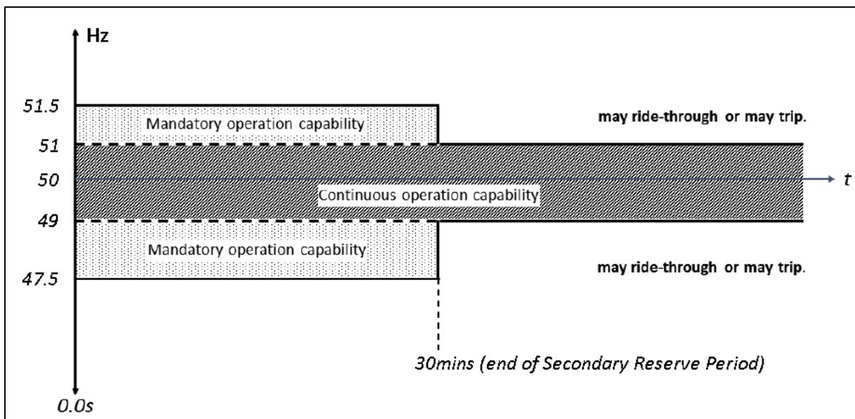
Figure 6.6 Frequency Ride-Through Requirements (adapted from IEEE 2800)
