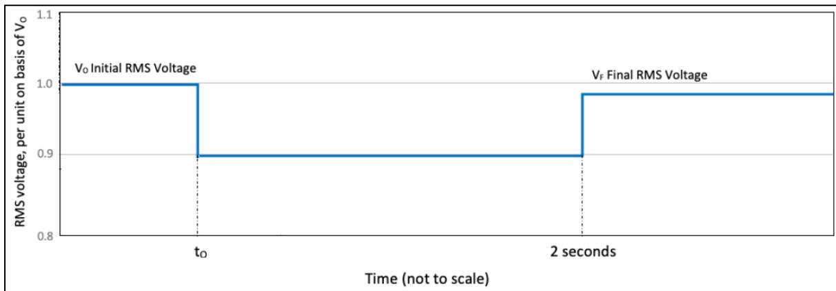
Figure 6.7 Minimum acceptable voltage due to infrequent events (adapted from IEEE 2800)
