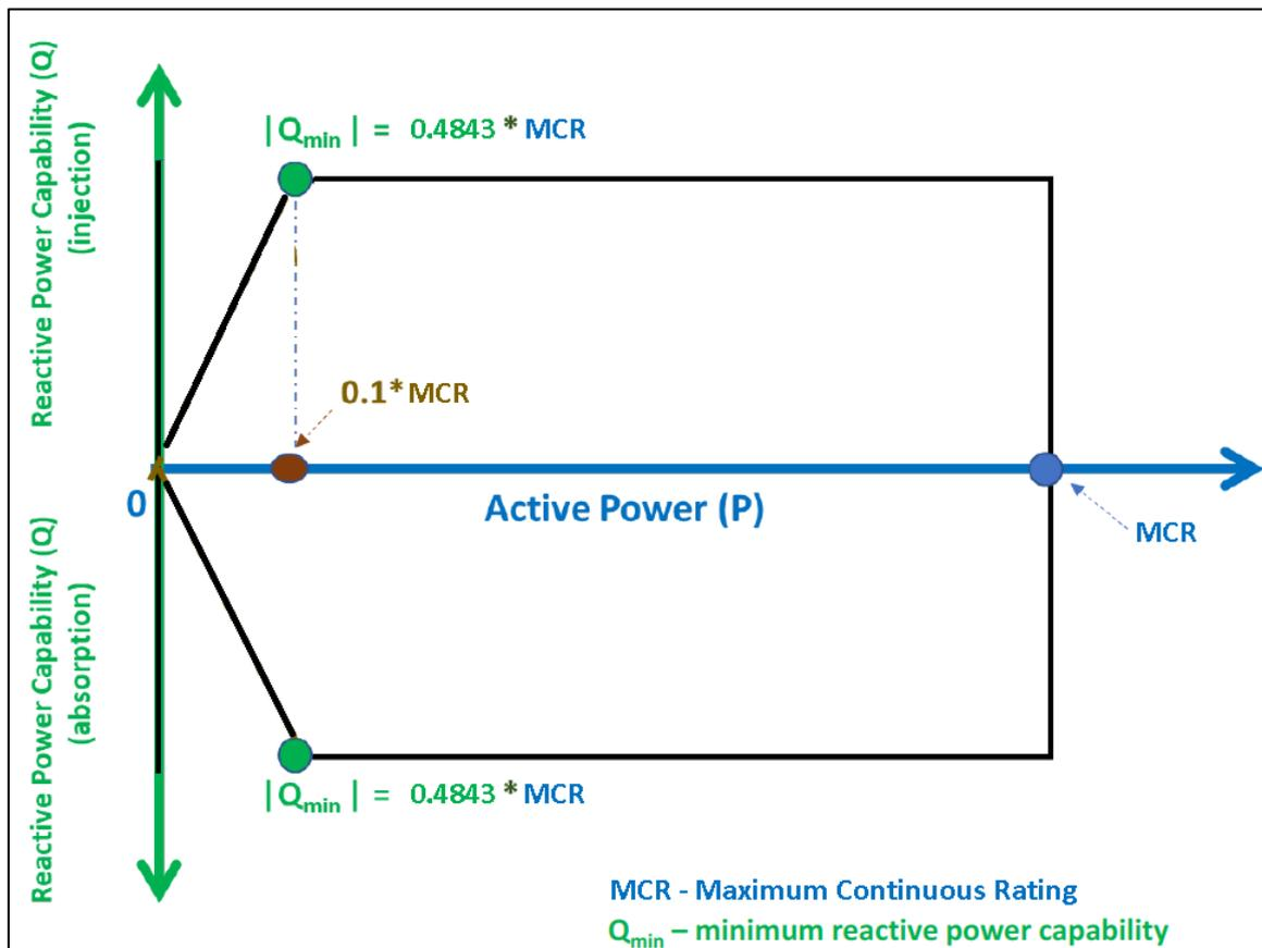
Figure 6.1 Minimum reactive power capability – Q versus P (adapted from IEEE 2800)
