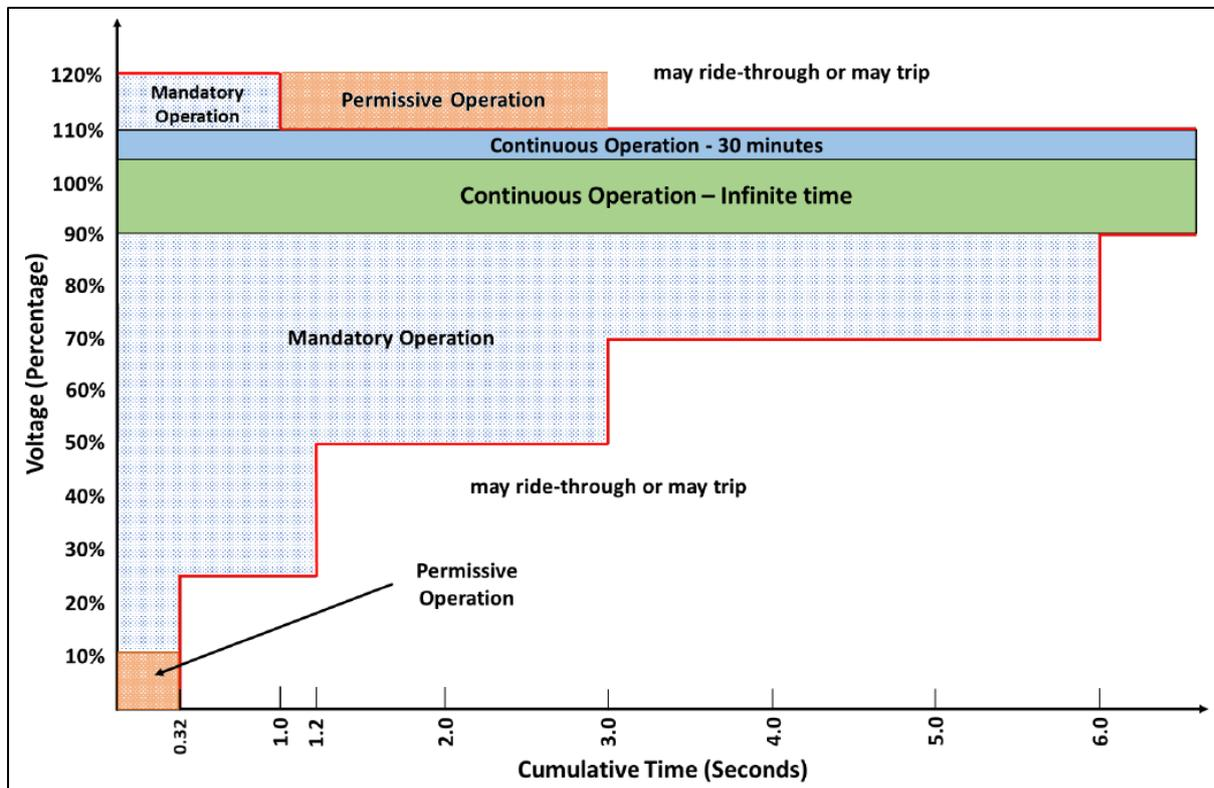
*Figure 6.4 Illustration of Voltage Ride-Through Requirements*
