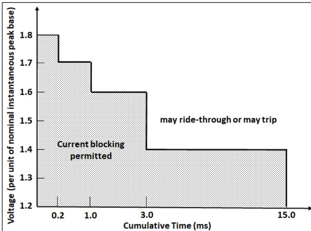
Figure 6.5 Transient overvoltage ride-through requirements (adapted from IEEE 2800)
