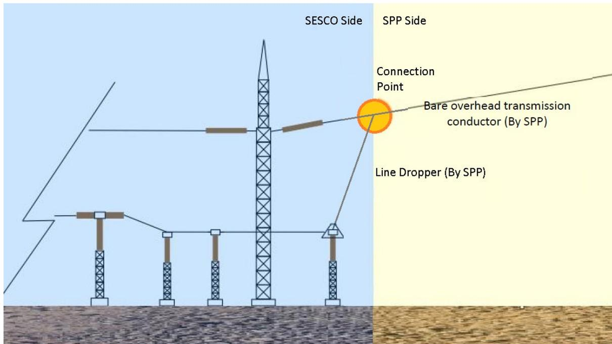
Figure 4.2 Connection Point at the connector of the down-dropper on the overhead line (OHL)
