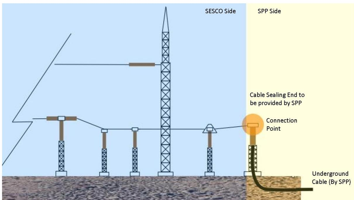
Figure 4.3 Connection Point at the connector of the Cable Sealing End on underground (U/G) cable
