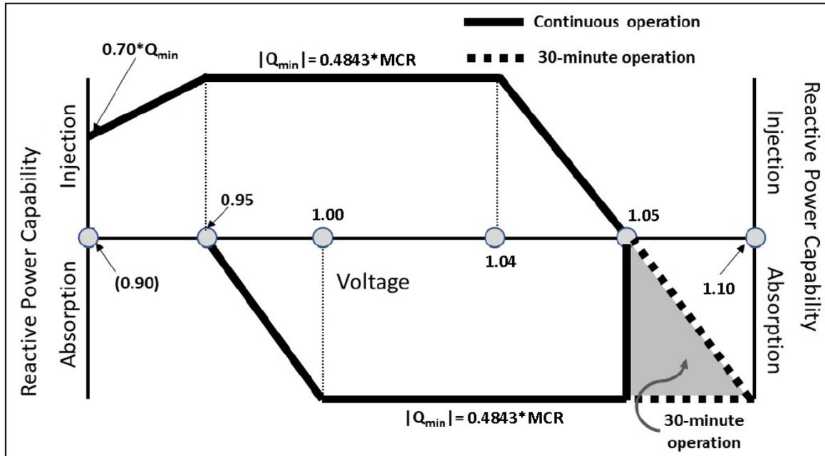
Figure 6.2 Minimum reactive power capability – Q versus V (adapted from IEEE 2800)
