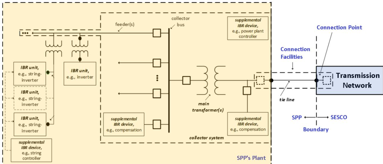
Figure 4.1 Example illustration of scope and asset demarcation (adapted from IEEE 2800)
